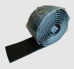
It is a triangular shaped elastomeric bitumen-rubber based super elastic chamfer tape used in the angulation of internal corners in the junction points of horizontal and vertical structural sections in accordance with the insulation.
